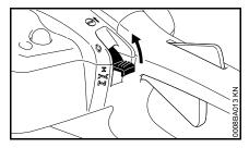
Move the Master Control lever in the direction of STOP or 0 – when released, the Master Control lever springs back to the normal run position I.
