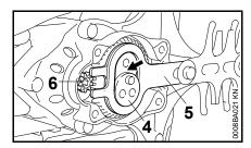
Squeeze grease into the gearbox housing (arrow) between the cam (4) and cutting blade (5) a little at a time (max. 5 g (1/5 oz)) while turning the drive pinion (6) with a
