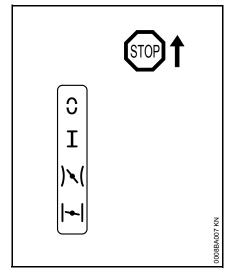
STOP or  ${\mathfrak O}$  – Master Control lever must be pushed in direction of STOP or  ${\mathfrak O}$  to switch off the ignition. When released, the Master Control lever springs back to the normal run position  ${\mathbf I}$  and the ignition is switched on again.
