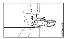
Carry the power tool by the handle – cutting blades behind you. Do not touch hot parts of the machine, especially the muffler and gear housing – **risk of burns!**
