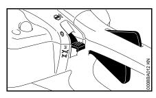
Press down the throttle trigger lockout and open the throttle – the Master Control lever moves to the
