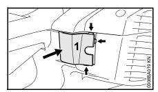
Close the flap (1), top first, then the bottom, tabs (arrows) must snap into position.
